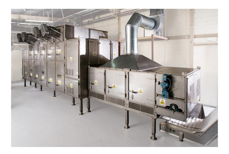
Bühler conveyor dryers, impingement ovens and hot-air expanders are efficient and sanitary solutions to high volume snack production. Thermal processing is used for direct expanded (DX) snacks, half-product pellets, confectionery products, coated snacks, baked potato chips and value-added snack products.
