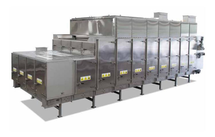
Bühler's Solis conveyor dryer has a unique dual plenum airflow that distributes heat and air uniformly to both sides of the product bed. This maximizes heat transfer to keep operating efficiency high and utility costs low. Independently controlled heating zones maximize processing flexibility and ensure the exact product specifications are met.
