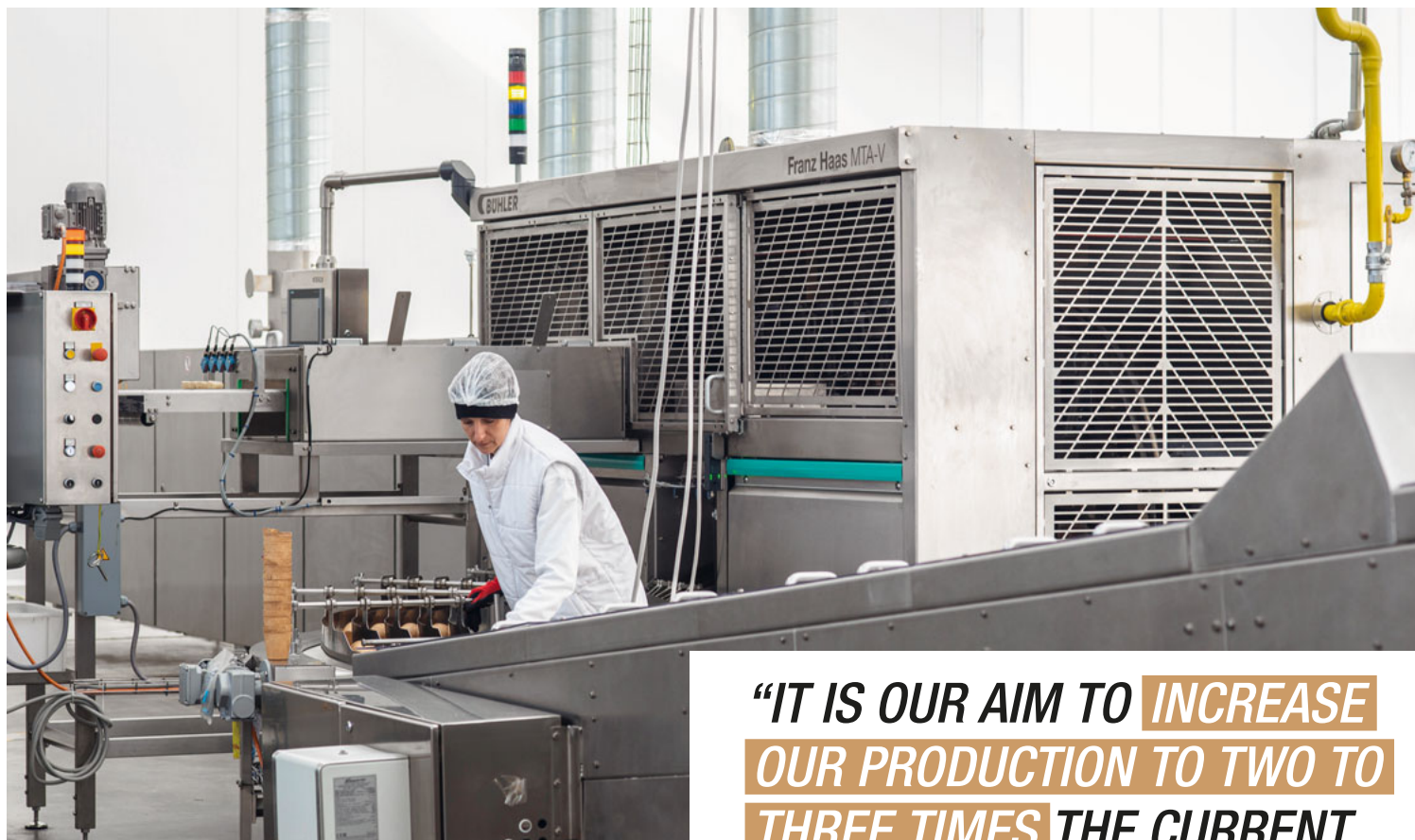
Bühler's Franz Haas MTA-V oven provided the industrial solution Cupffee needed to increase capacity. It produces around 3,400 cups an hour.
